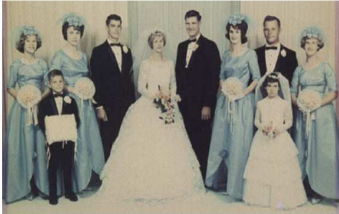
Displayed 1968 Ektacolor print with severe magenta dye fading and loss of detail in skin tones and in the bride's dress while the groom's black tuxedo appears unaffected.
